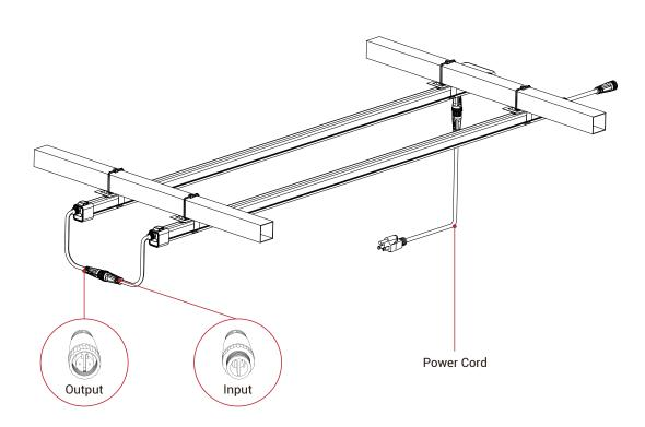
3. To daisy-chain multiple clone light bars, position the input of one fixture right next to the output of the next. Remove the protection cover, then connect and lock the input and output together.
