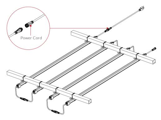
A single power source can connect and power up to 90 clone light bars in a daisy chain configuration. Once daisy-chained, connect the 120V power cord to the power source to energize all fixtures.
