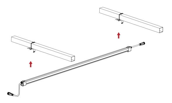
2. Lock the fixture securely into both steel clips.
