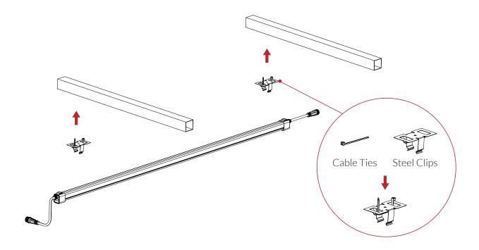
1. Securely fasten the steel clips to a fixed, solid ceiling structure (e.g., unistrut, grow rack). Ensure the clips are positioned no more than 4 feet apart.
